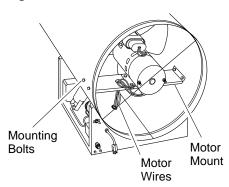
Figure 7 - Location of Fan and Motor
